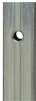
Rail (unloaded) with CZS coating – after 99 hours of salt spray test (according to DIN EN ISO 9227)
