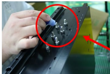
Fig. 5.15: Use non-magnetic tool to install the stator
